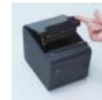
Step 1: Pull up the lever, and open the door until it is fully open.
